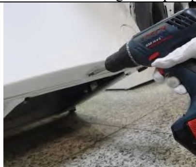
3.6. Tighten the screw fixing the front panel at the bottom
