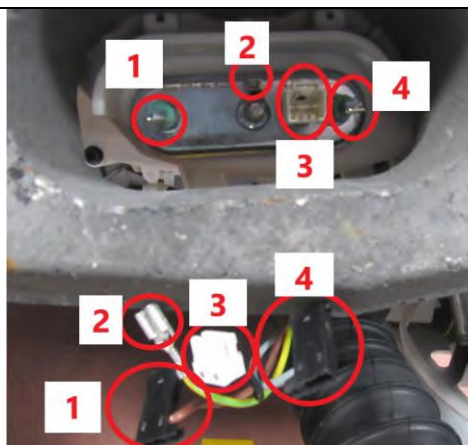
3.2. Fit the heater to the house well
