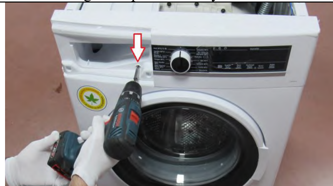
3.11.2 Tighten the screw which fixes the control panel to the front panel.
