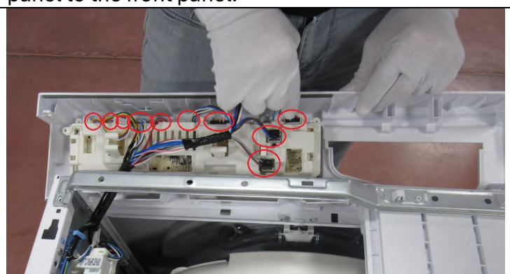
2.4.1 Remove the sockets on the card
