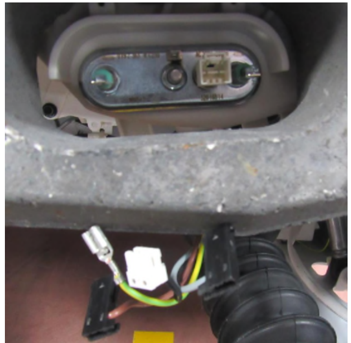
Remove the heater sockets
