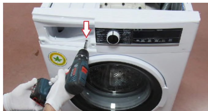
4.13 Tighten the screw which fixes the control panel to the front panel.
