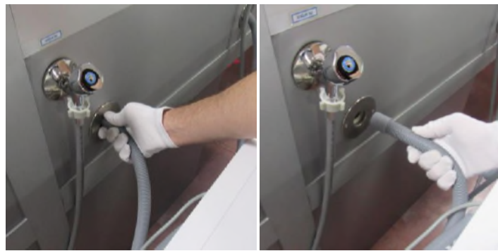
Disconnect the drain hose
