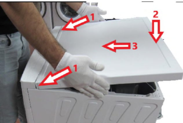
4.16 Fit the upper tray according to movement above
