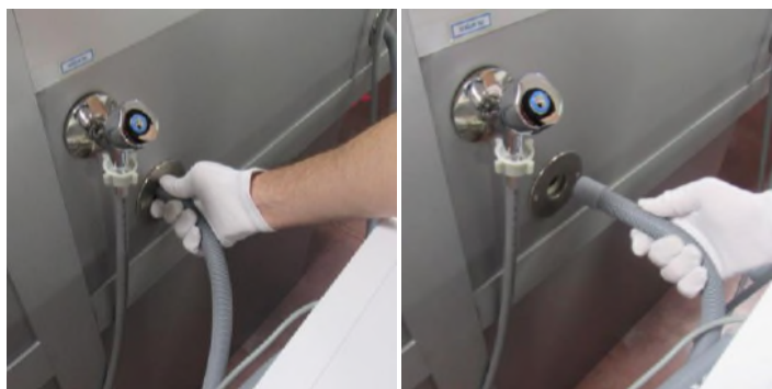
1.3 Disconnect the drain hose
