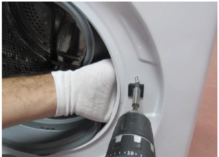
4.6 Tighten the door lock screw
