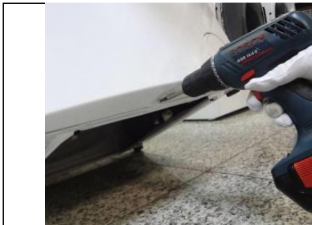
2.8. Remove the screw fixing the front panel at the bottom.
