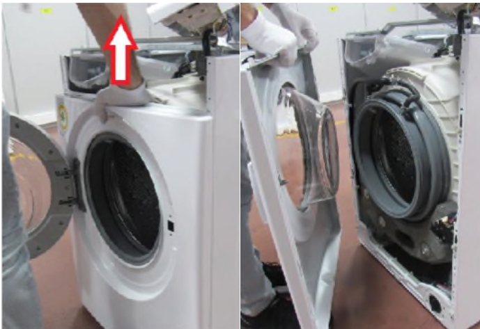
3.12 Pull up and remove the front panel.
