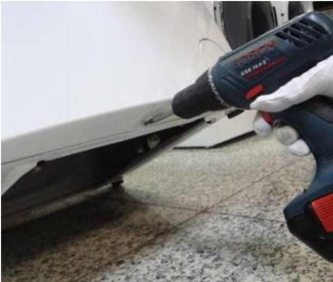
Remove the screw fixing the front panel at the bottom.
