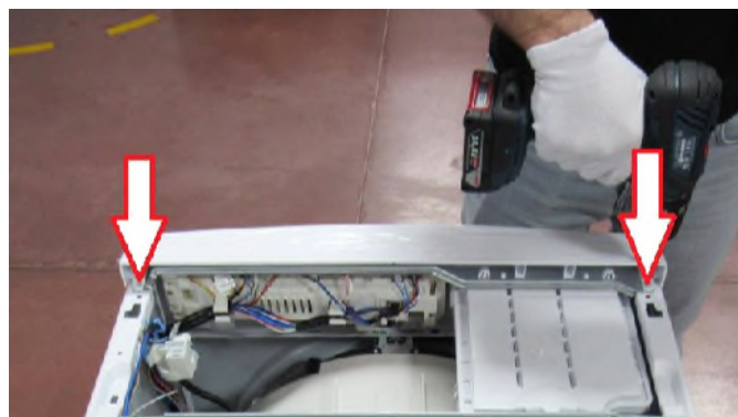
4.12 Tighten two screws fixing control panel.
