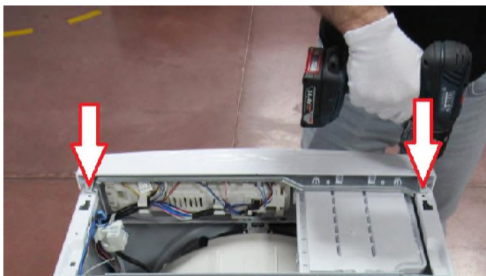
3.5 Remove two screws fixing control panel.
