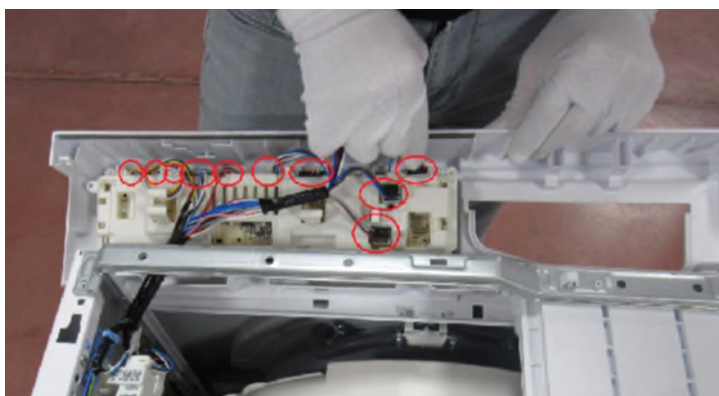
3.6 Remove the sockets on the card.
