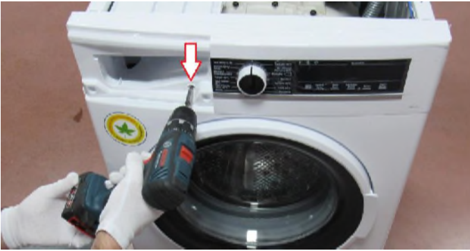
3.4 Remove the screw which fixes the control panel to the front panel.
