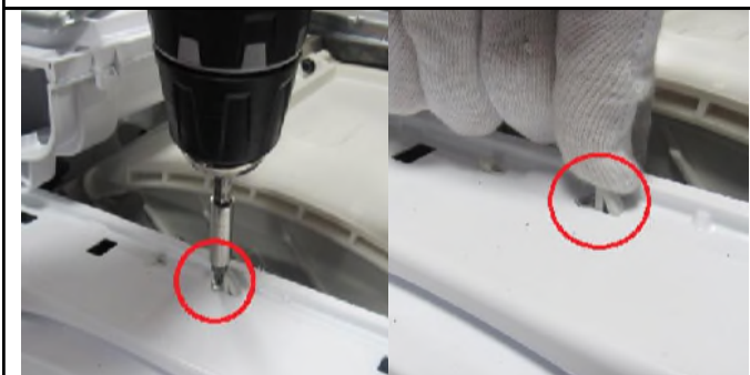
2.5. Remove the screw fixing twinjet elbow.
