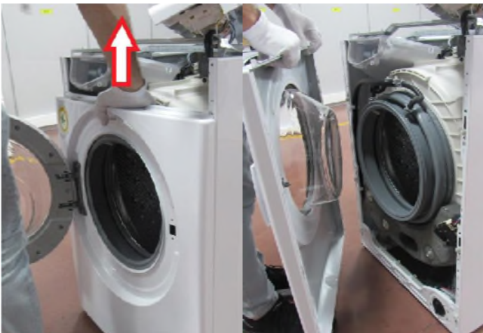
Pull up and remove the front panel.
