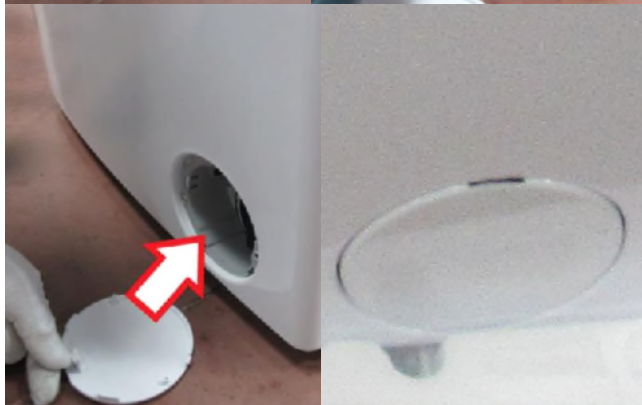
4.9 Fit the screw and plastic part located under the pump cover
