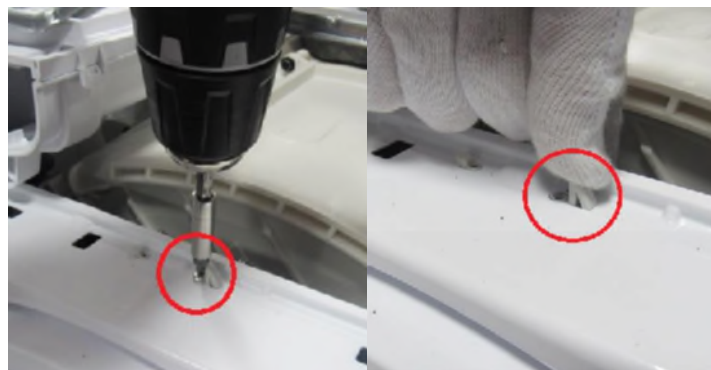
4.10 Assemble the twinjet elbow to the front panel
