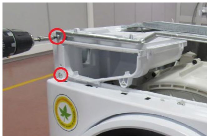
4.11 Tighten the screw on support bracket and two screws fixing front panel to body
