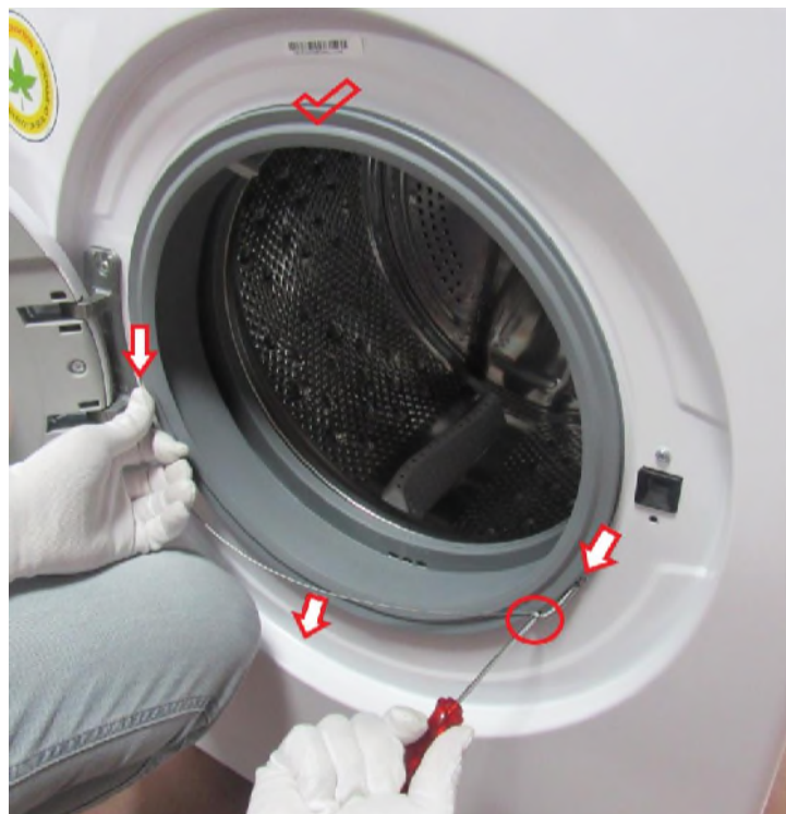
4.3 Fix the tub bellow seal and fix the wire by using the small screwdriver
