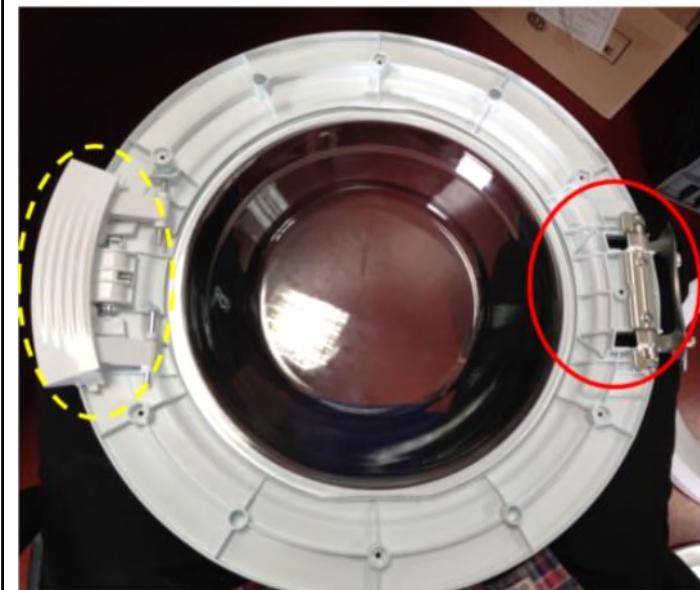
2.7. Remove the plastic parts as shown in the photo above.
