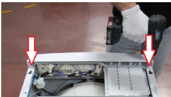
Remove two screws fixing control panel.
