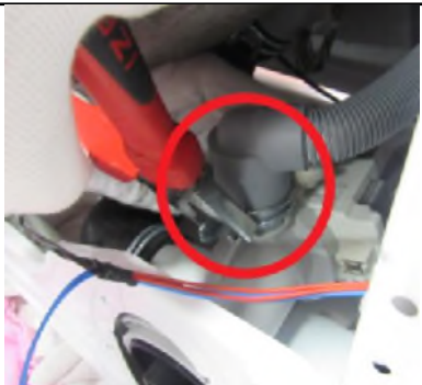
2.14. Remove clamp holding drain hose by using a plier.
