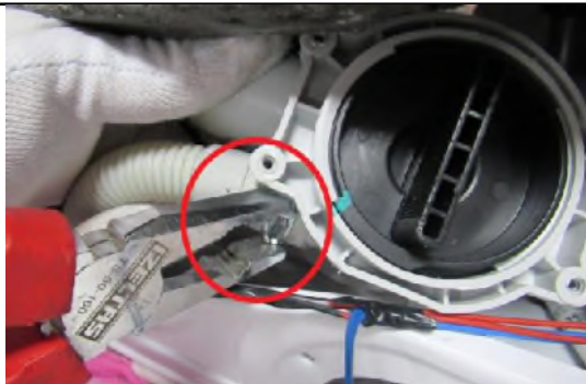
2.15. Remove clamp holding twinjet hose by using a plier.
