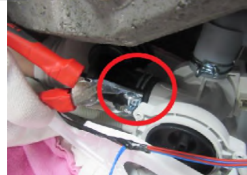
2.13. Remove clamp fixing tub outlet hose by using a plier
