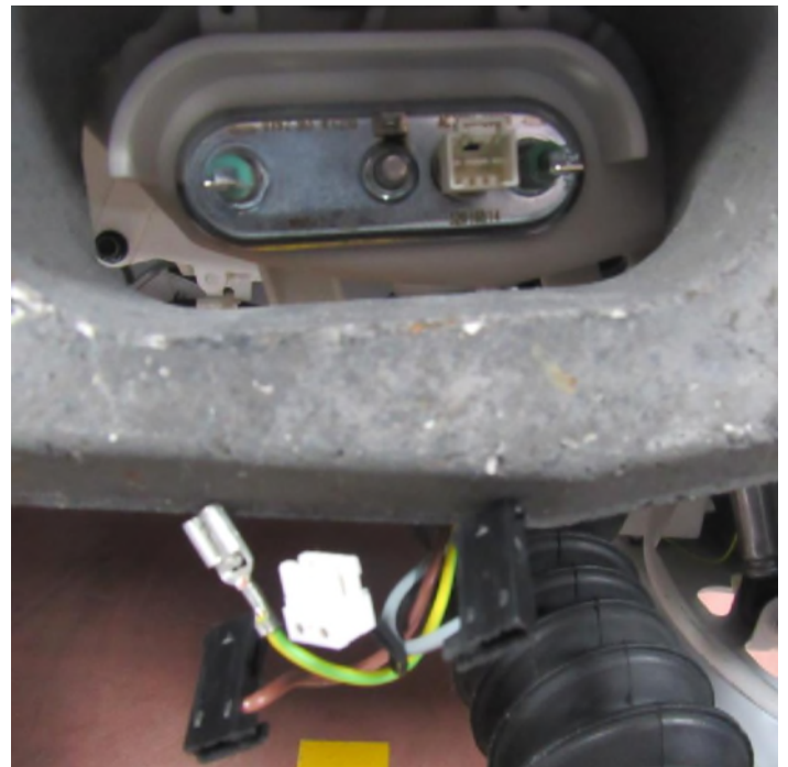
Remove the heater sockets
