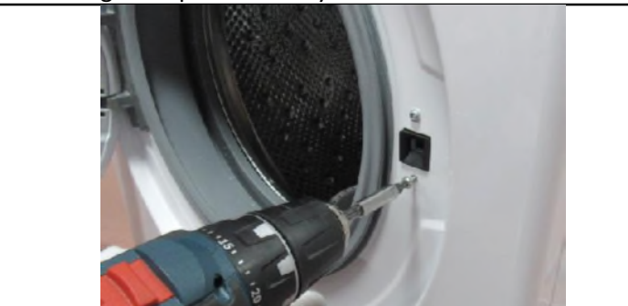
2.6. Remove the screws fixing the door lock.
