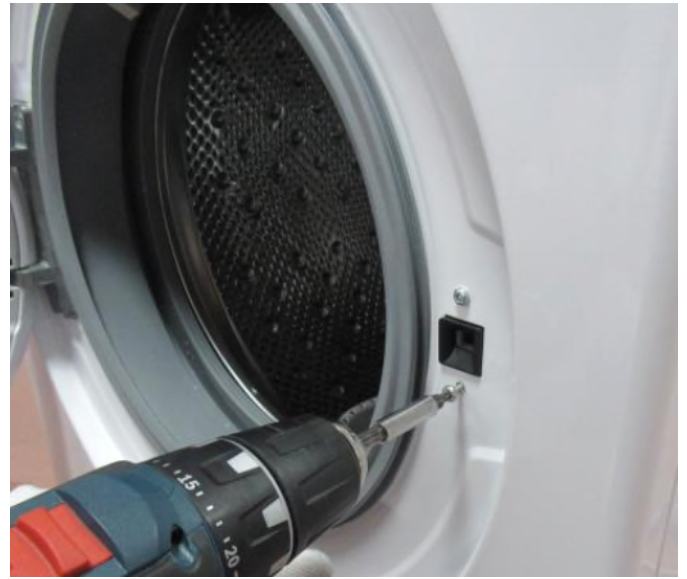
3.1 Remove the screws fixing the door lock.
