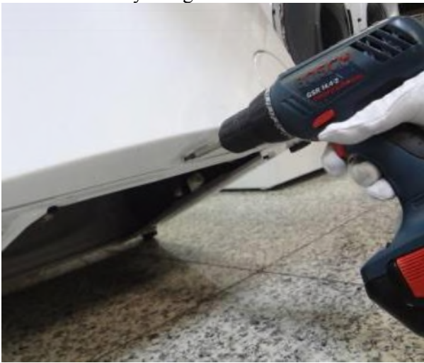
4.8 Tighten the screw fixing the front panel at the bottom
