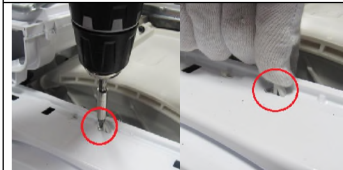
2.5. Remove the screw fixing twinjet elbow.
