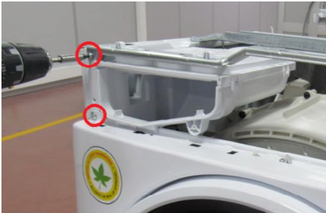
3.6 Remove the screw on support bracket and two screws fixing front panel to body
