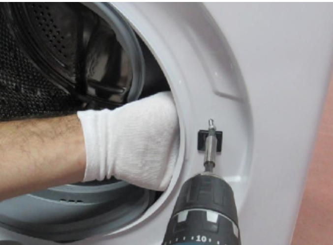
Tighten the door lock screw
