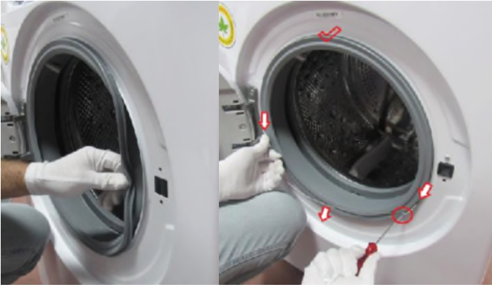
4.7 Pull the tub bellow seal to the outside and assemble the wire by using small screwdriver
