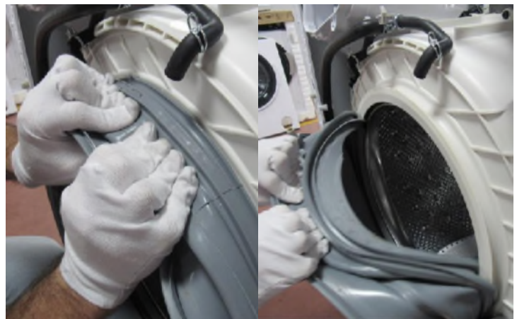
3.15 Hold the tub bellows seal and gasket-body fixing spring together, and pull them out.
