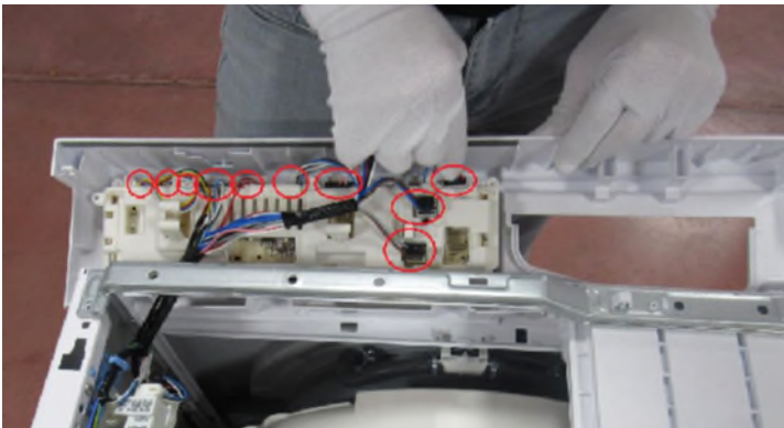
3.6 Remove the sockets on the card.
