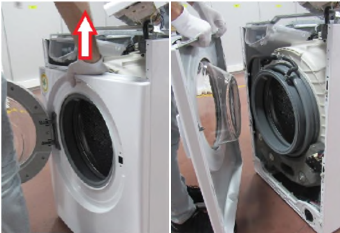
3.12 Pull up and remove the front panel.
