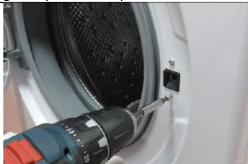
2.6. Remove the screws fixing the door lock.
