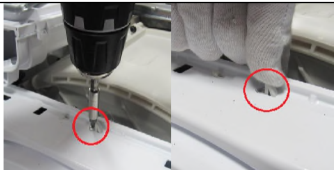
2.5. Remove the screw fixing twinjet elbow.
