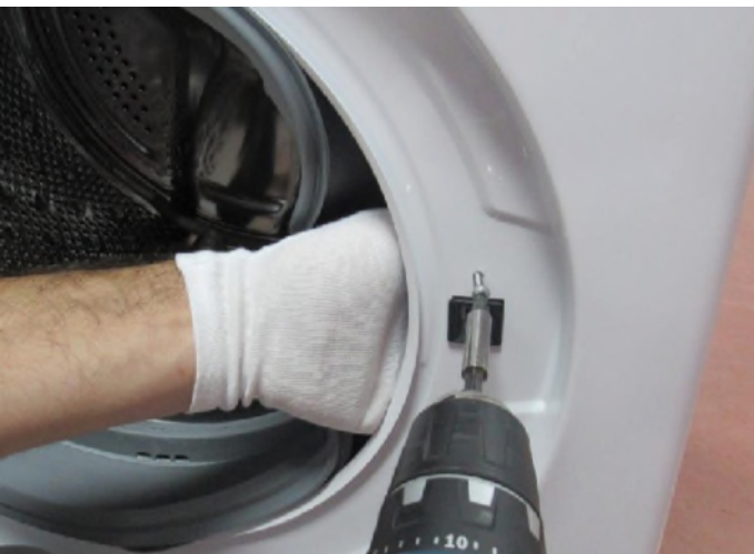
Tighten the door lock screw
