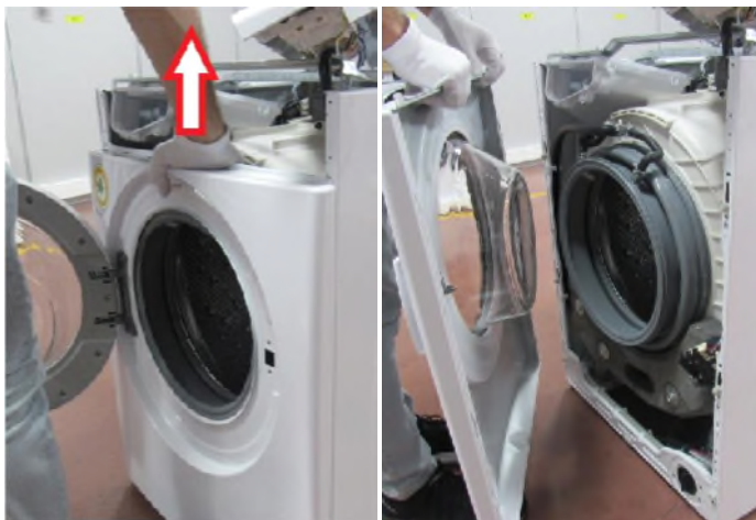
3.12 Pull up and remove the front panel.
