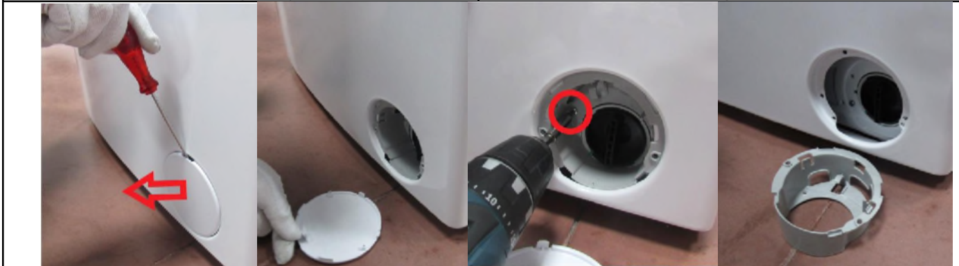
2.7. Remove the screw and plastic part located under the pump cover
