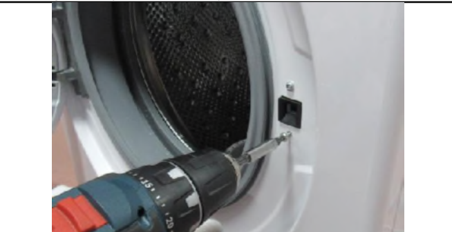
2.6. Remove the screws fixing the door lock.
