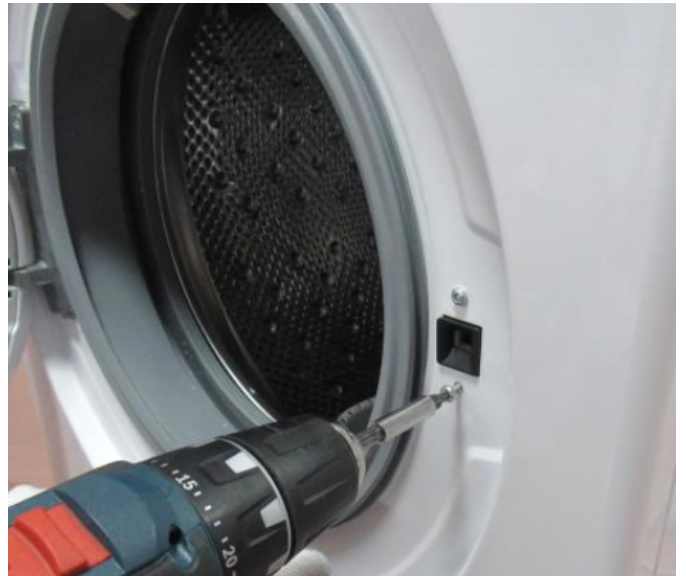
3.1 Remove the screws fixing the door lock.
