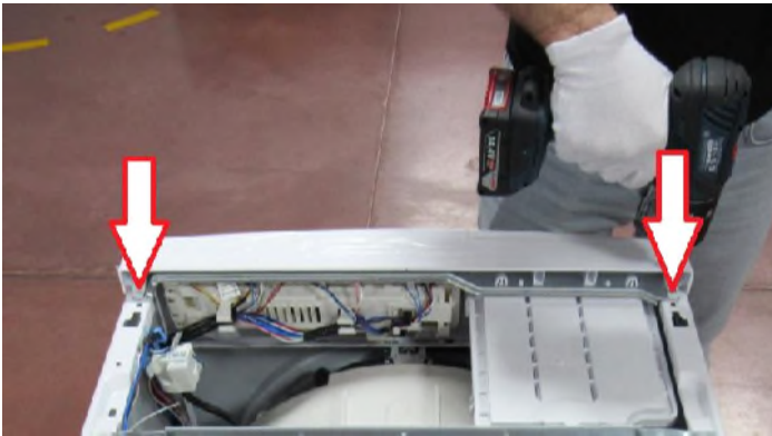
4.4 Tighten the two screws on control panel.
