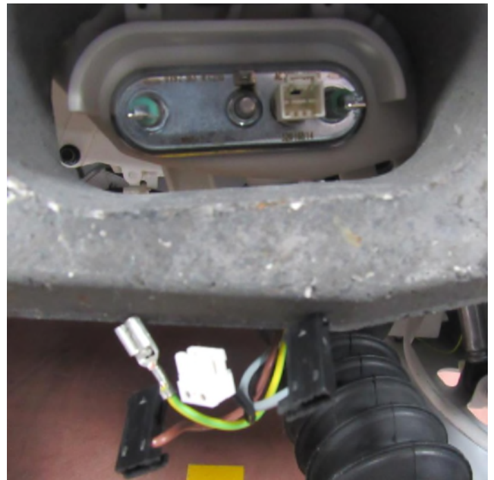
Remove the heater sockets
