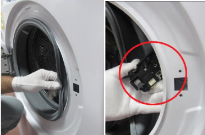
3.3 Remove the right side of the tub bellows seal and reach to door lock
