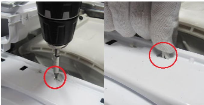
3.7 Remove the screw fixing twinjet elbow.
