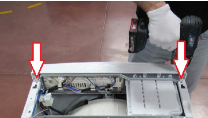
4.4 Tighten the two screws on control panel.
