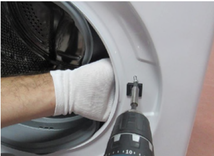
Tighten the door lock screw
