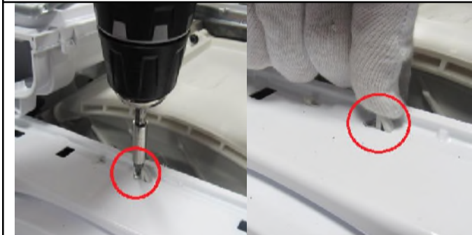
2.5. Remove the screw fixing twinjet elbow.
