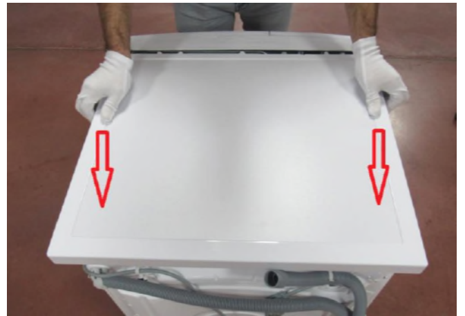
3.2 Push the top-plate back and pull it up.
