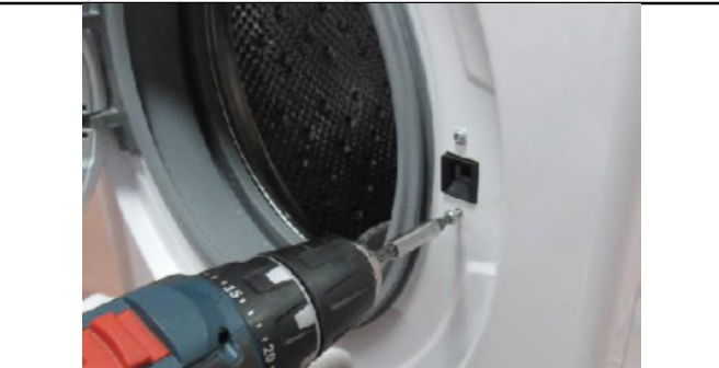
2.6. Remove the screws fixing the door lock.
