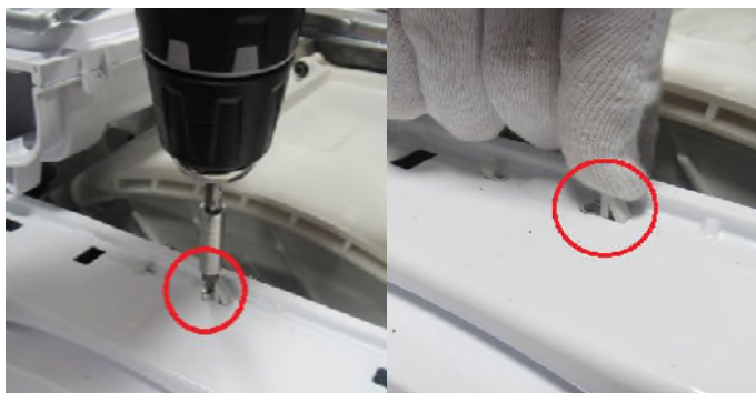
3.7 Remove the screw fixing twinjet elbow.
