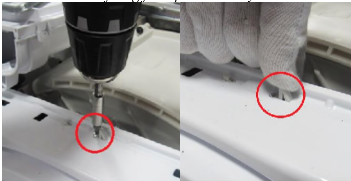
Remove the screw fixing twinjet elbow.
