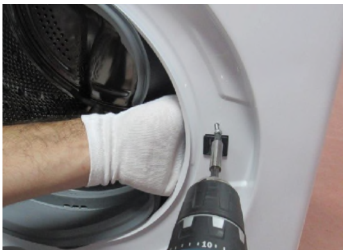
Tighten the door lock screw
