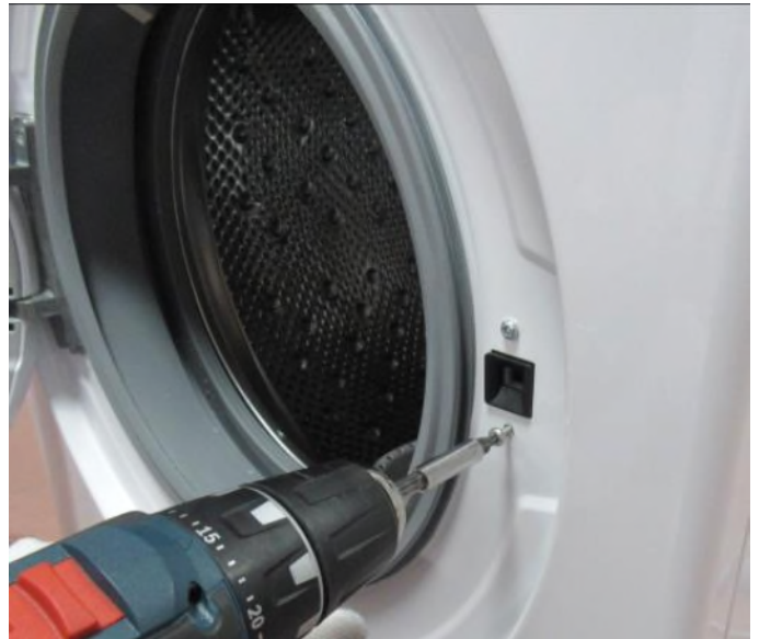
3.8 Remove the screws fixing the door lock.
