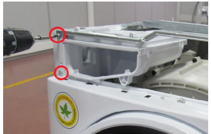
4.11 Tighten the screw on support bracket and two screws fixing front panel to body
