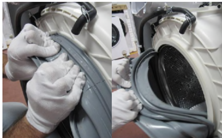
3.15 Hold the tub bellows seal and gasket-body fixing spring together, and pull them out.
