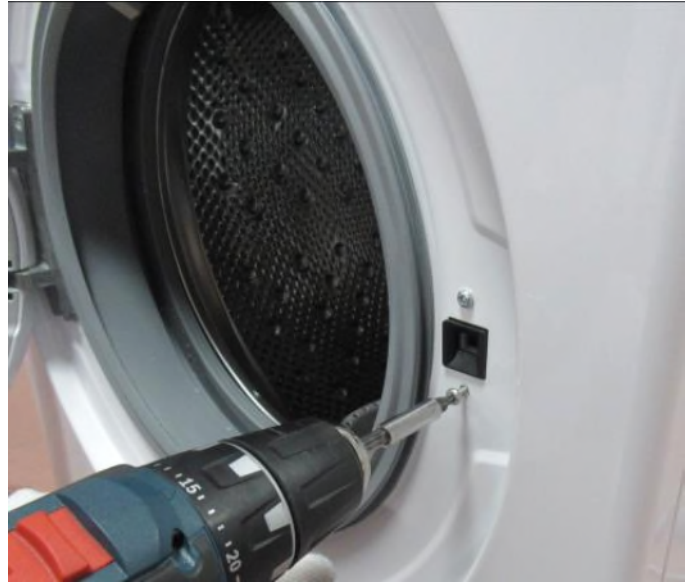
3.8 Remove the screws fixing the door lock.
