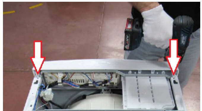
4.12 Tighten two screws fixing control panel.
