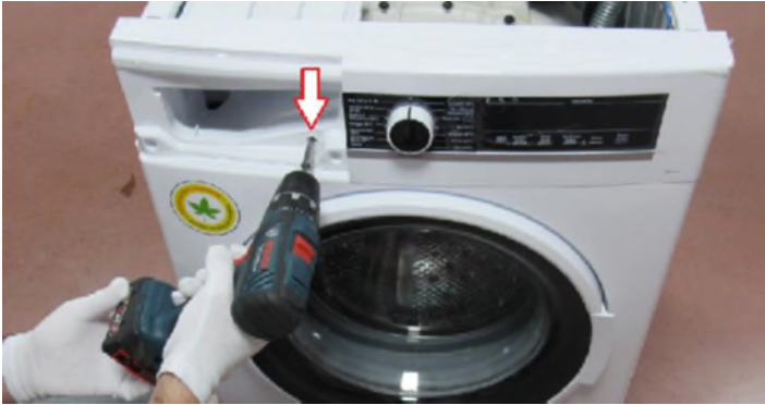
Remove the screw which fixes the control panel to the front panel.
