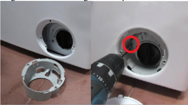
4.8 Tighten the screw fixing the front panel at the bottom
