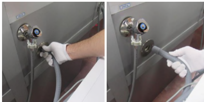
1.3 Disconnect the drain hose
