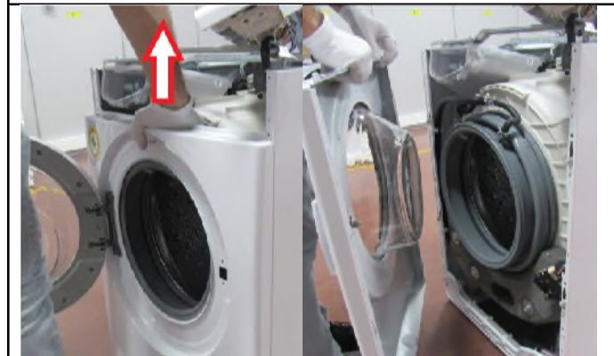
2.10. Pull up and remove the front panel.
