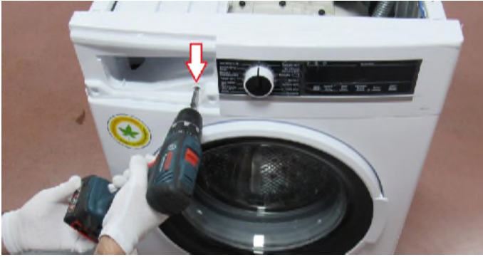
3.4 Remove the screw which fixes the control panel to the front panel.
