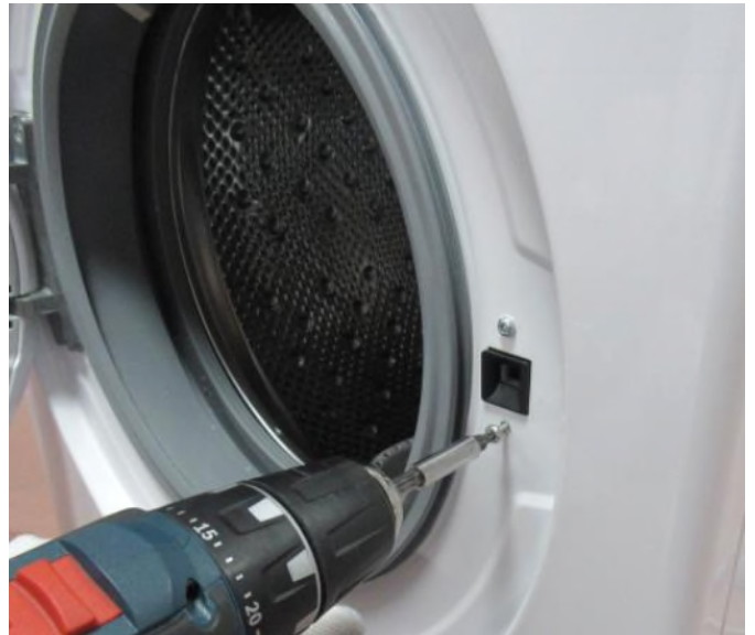
3.1 Remove the screws fixing the door lock.
