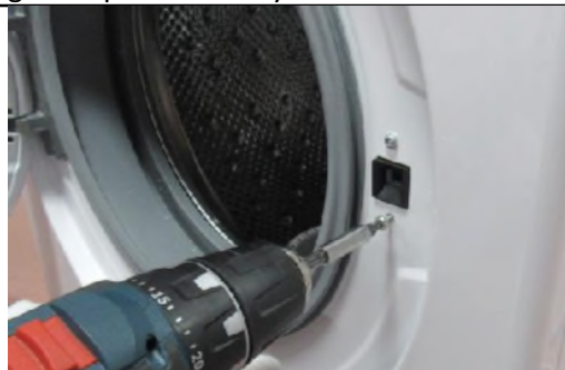
2.6. Remove the screws fixing the door lock.
