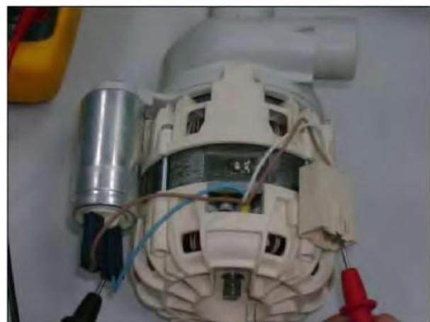
Measurement of the secondary windings of the washing pump (white cable – blue cable) (117.9-135.6 Ω)
