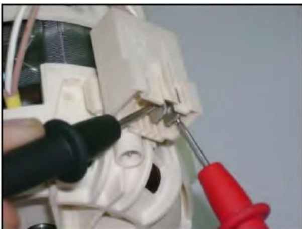
Measurement of the primary windings of the washing pump. (118.2-135.9 Ω)
