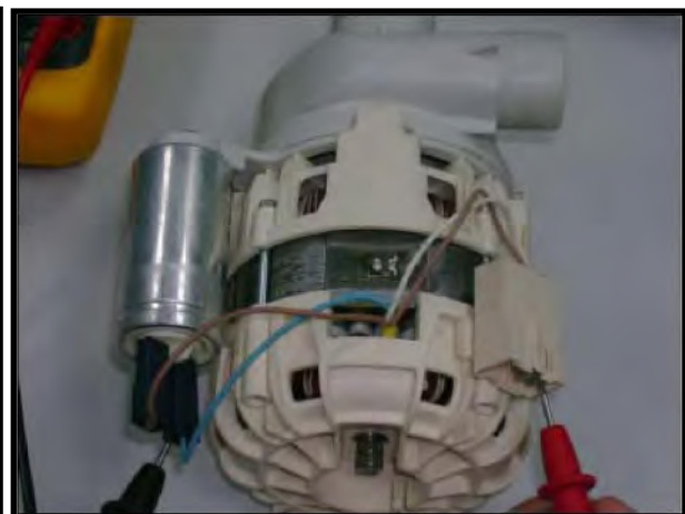
Measurement of the secondary windings of the washing pump (white cable – blue cable)
