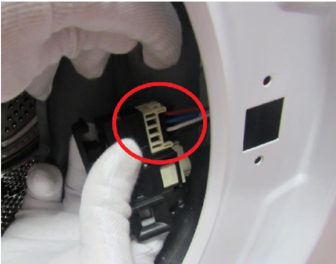
4.1 Unplug the connector and remove the door lock. Connect the new door lock to connector.
