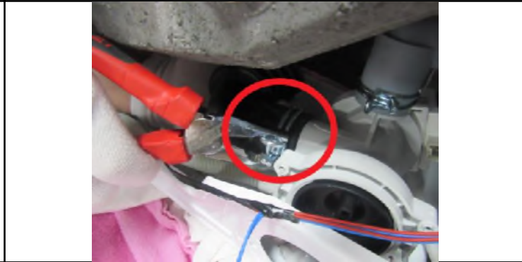
2.13. Remove clamp fixing tub outlet hose by using a plier
