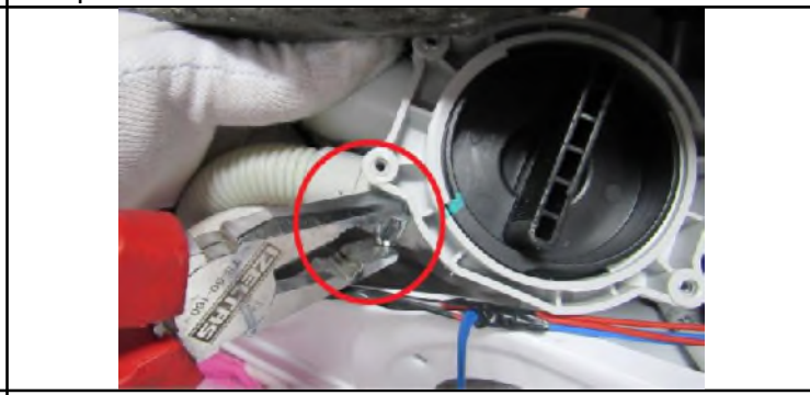
2.15. Remove clamp holding twinjet hose by using a plier.
