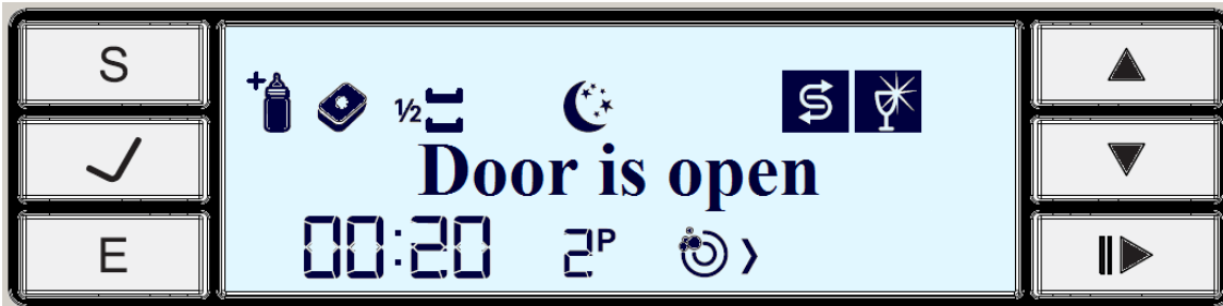
After the door is opened (Note: without S/P button pressed, remaining program icons do not become ON)
