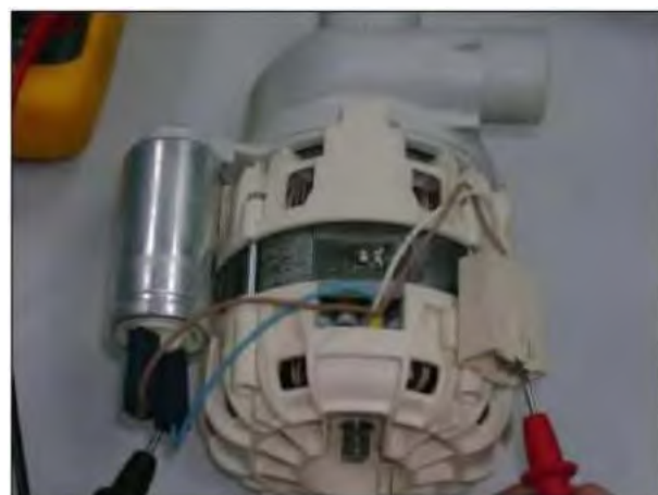
Measurement of the secondary windings of the washing pump (white cable – blue cable) (117.9-135.6 \Omega )
