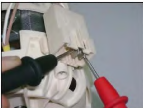
Measurement of the primary windings of the washing pump. (118.2-135.9 \Omega )
