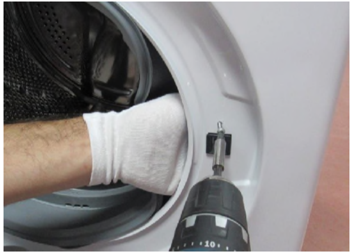
4.6 Tighten the door lock screw
