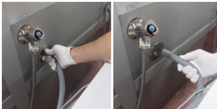
1.3 Disconnect the drain hose
