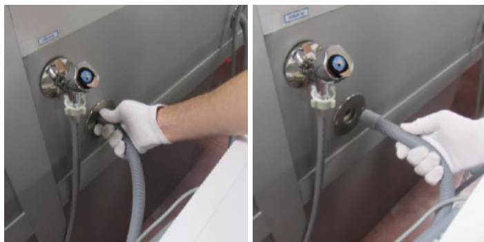
Disconnect the drain hose
