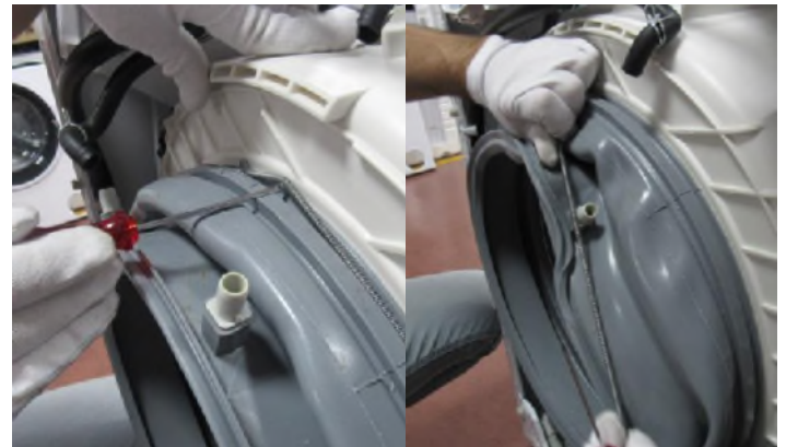
3.14 Remove the tub gasket clip by using small screwdriver.
