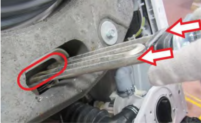
3.1. Place the heater to the guide wire in the front tub and push it
