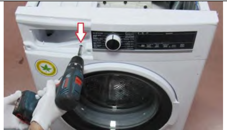
3.11. Tighten the screw which fixes the control panel to the front panel.
