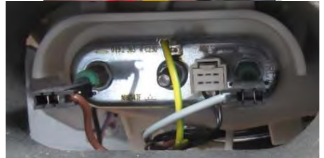
3.4. Connect the all sockets on the heater
