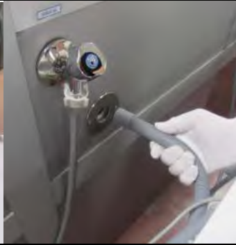
1.2 Turn off the tap and disconnect the hose from the valve
