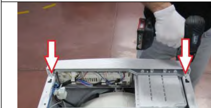
3.12 Tighten two screws fixing control panel.
