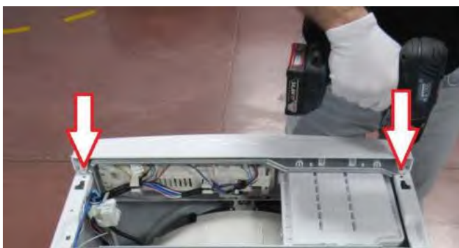
2.3.2 Remove two screws fixing control panel and disassemble the control panel
