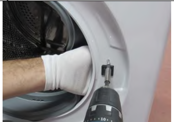
3.5.1 Tighten the door lock screw
