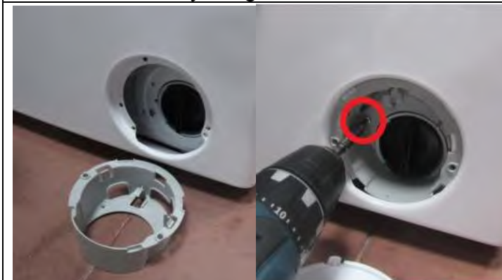
3.8.1 Fit the screw and plastic part located under the pump cover
