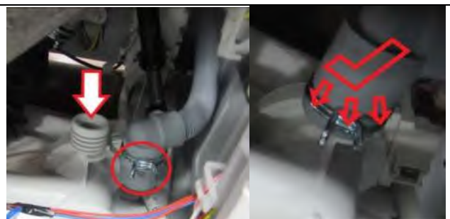
3.2. Connect the drain hose by using a plier to fix the clamp
