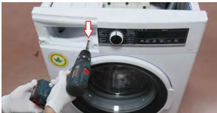
3.5. Tighten the screw which fixes the control panel to the front panel.
