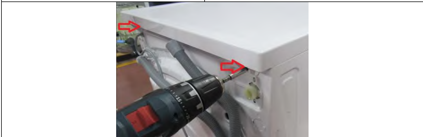
3.14. Tighten two screws that fix the top-plate at the back
