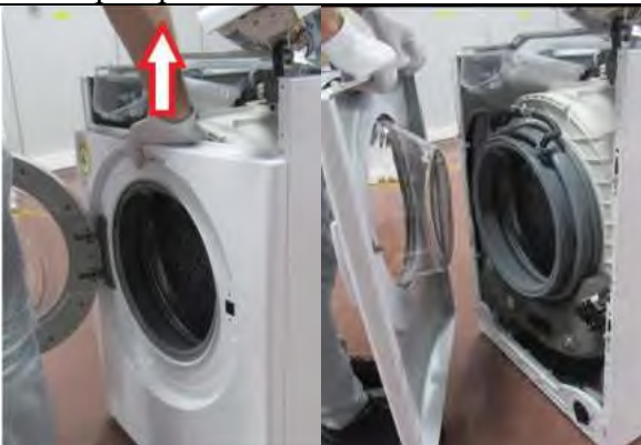
2.7.2 Pull up and remove the front panel.
