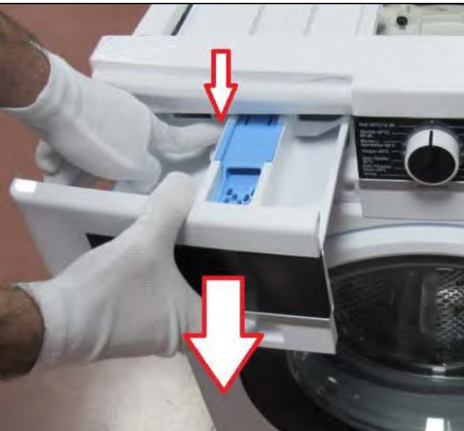
2.2.1 While pressing siphon cover keep pulling drawer to remove it.
