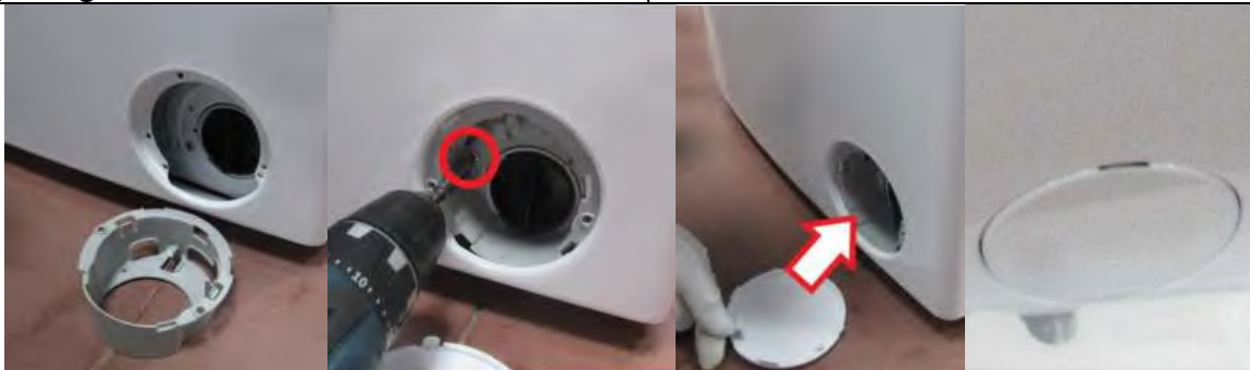
3.9. Tighten the screw and plastic part located under the pump cover
