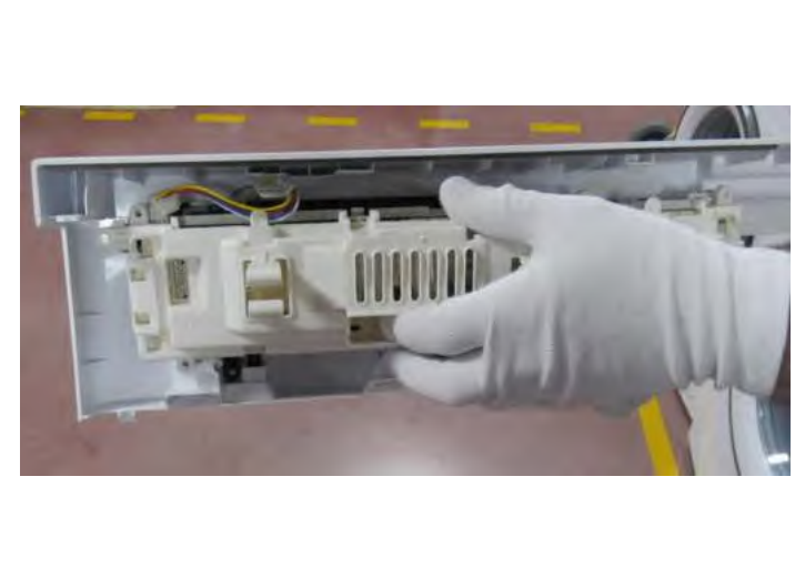
3.2. Push the PCB box and fit to the housing
