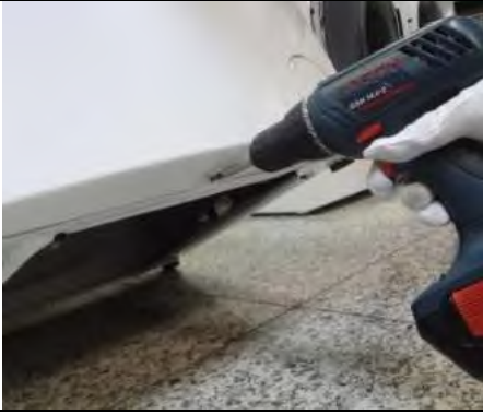
2.4.2 Remove the screw fixing the front panel at the bottom.
