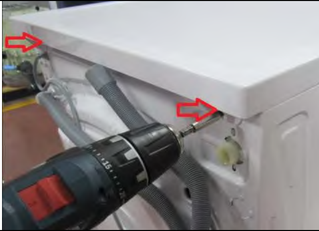
3.16 Tighten two screws that fix the top-plate at the back.
