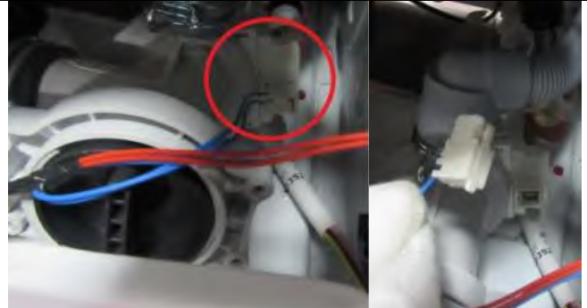
2.10.1 Remove the drain pump connector
