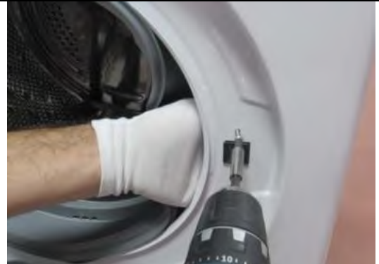
3.6. Tighten the door lock screw
