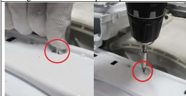
3.10. Assemble the twinjet elbow to the front panel
