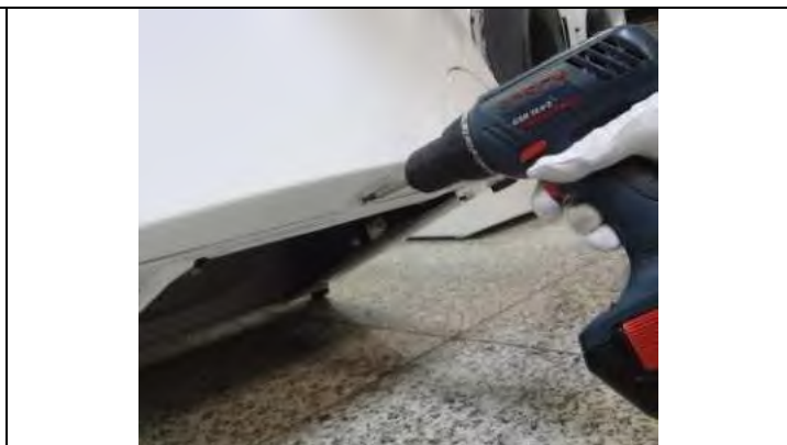
3.7.1 Tighten the screw fixing the front panel at the bottom
