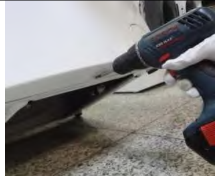
3.6. Tighten the screw fixing the front panel at the bottom
