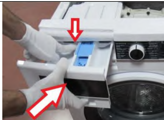
3.6. While pressing siphon cover keep pushing drawer to assemble it.
