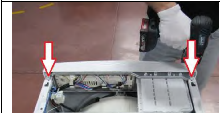
3.11.1 Tighten two screws fixing control panel.
