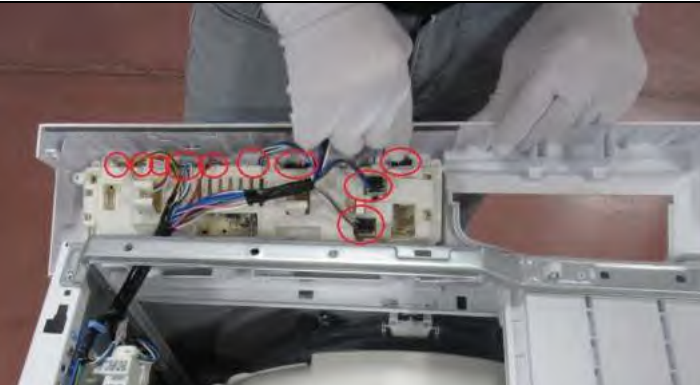
2.4.1 Remove the sockets on the card
