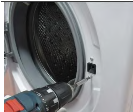
2.1 Remove the screws fixing the door lock
