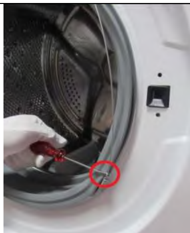
2.2 Remove the wire by using small screwdriver
