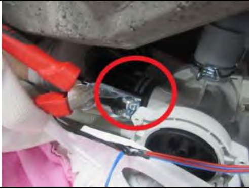
2.9.1 Remove clamp fixing tub outlet hose by using a plier
