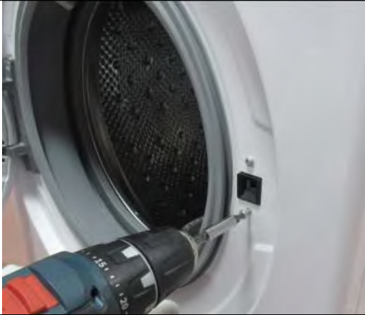
2.4.4 Remove the screws fixing the door lock.
