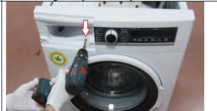
3.11.2 Tighten the screw which fixes the control panel to the front panel.
