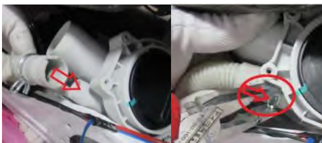
3.1. Connect the twinjet hose by using a plier to fix the clamp
