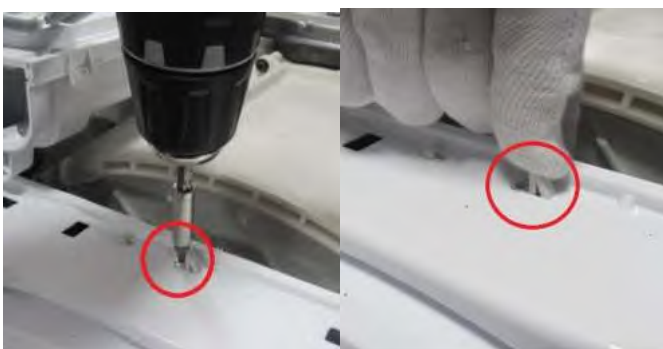
3.7. Tighten the screw and plastic part located under the pump cover
