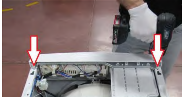
3.4 Tighten the two screws on control panel.
