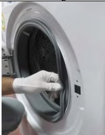
2.3 Remove the right side of the tub bellows seal
