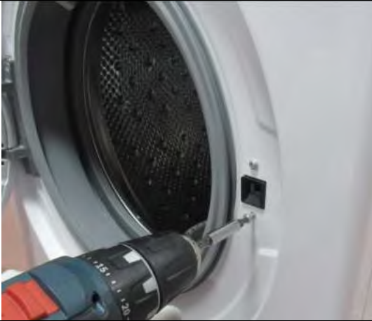
2.4.4 Remove the screws fixing the door lock.
