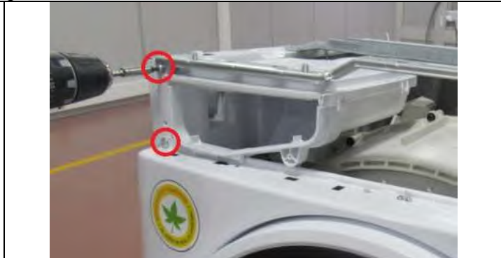
3.10.1 Tighten the screw on support bracket and two screws fixing front panel to body
