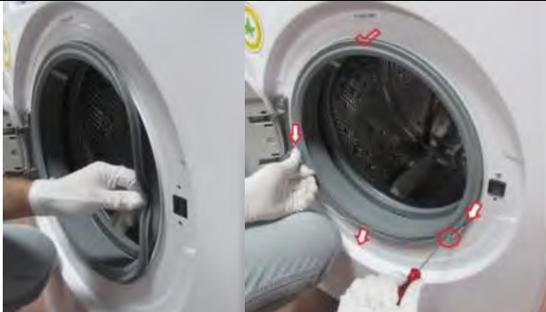
3.5. Pull the tub bellow seal to the outside and assemble the wire by using small screwdriver
