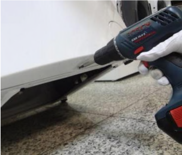
3.10 Remove the screw fixing the front panel at the bottom.
