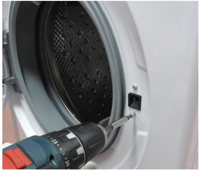
3.1 Remove the screws fixing the door lock.
