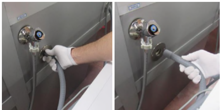
1.3 Disconnect the drain hose
