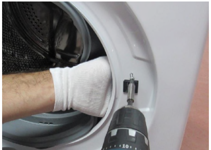
4.6 Tighten the door lock screw
