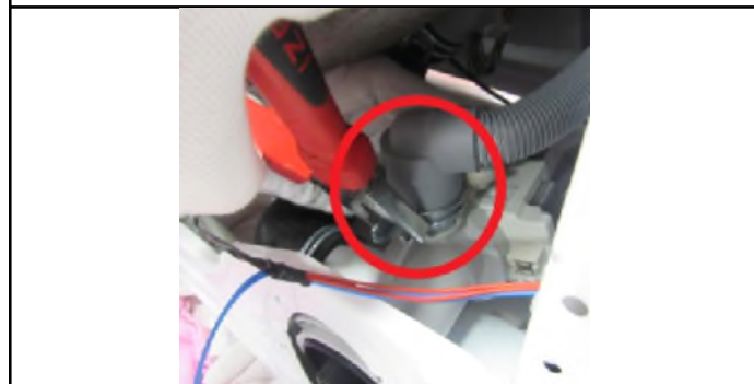
2.14. Remove clamp holding drain hose by using a plier.
