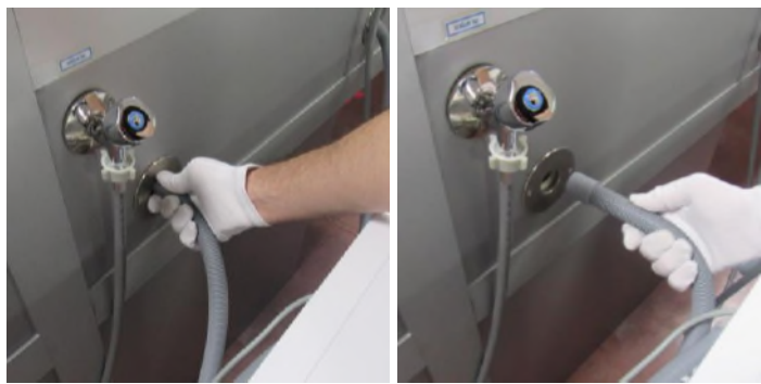
1.3 Disconnect the drain hose
