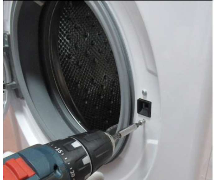
Remove the screws fixing the door lock.
