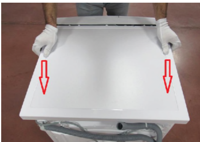
2.2. Push the top-plate back and pull it up.
