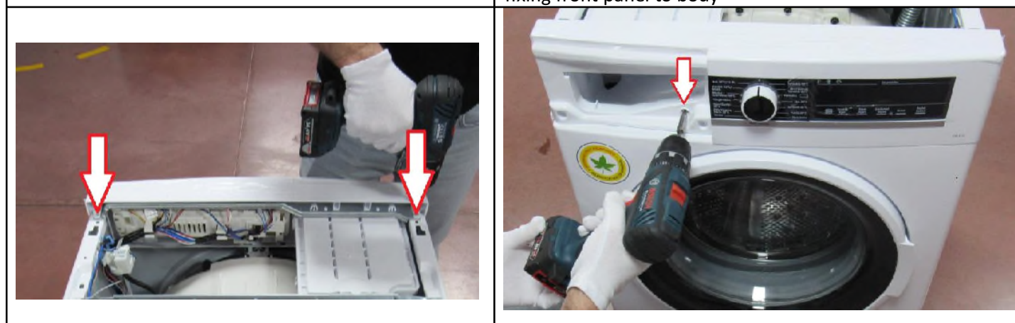
3.11. Tighten the screw which fixes the control panel to the front panel.
