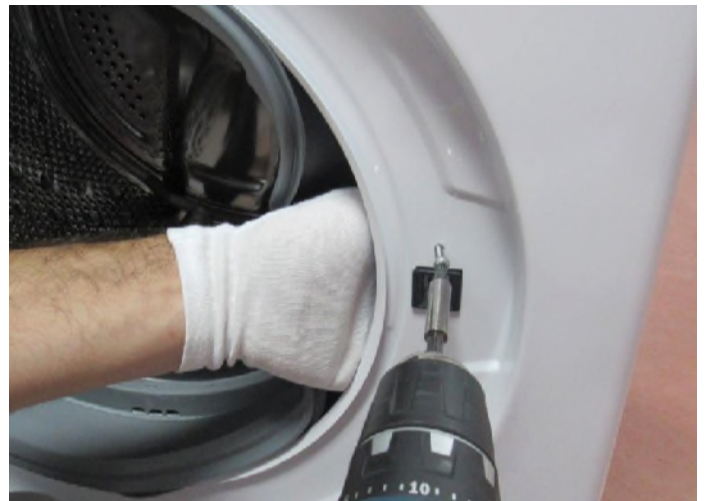
4.6 Tighten the door lock screw
