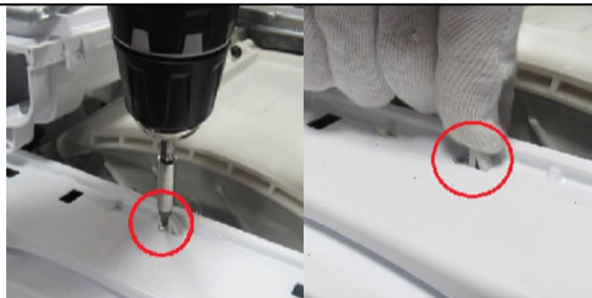
2.5. Remove the screw fixing twinjet elbow.
