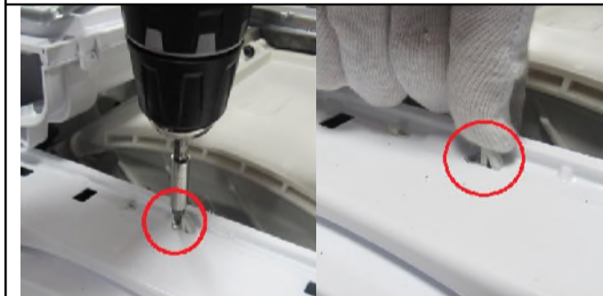
2.5. Remove the screw fixing twinjet elbow.
