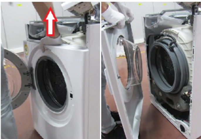
3.12 Pull up and remove the front panel.
