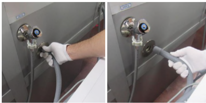
Disconnect the drain hose
