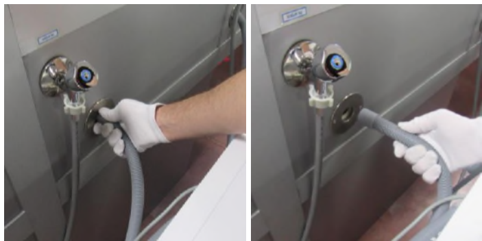
1.3 Disconnect the drain hose
