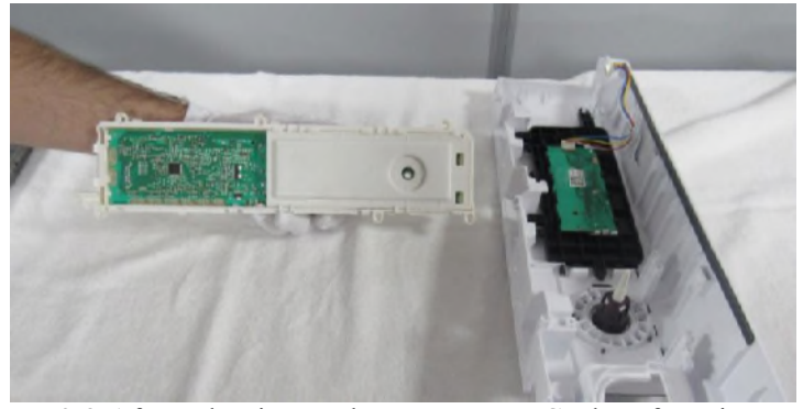
3.8 After releasing sockets, remove PCB box from its housing
