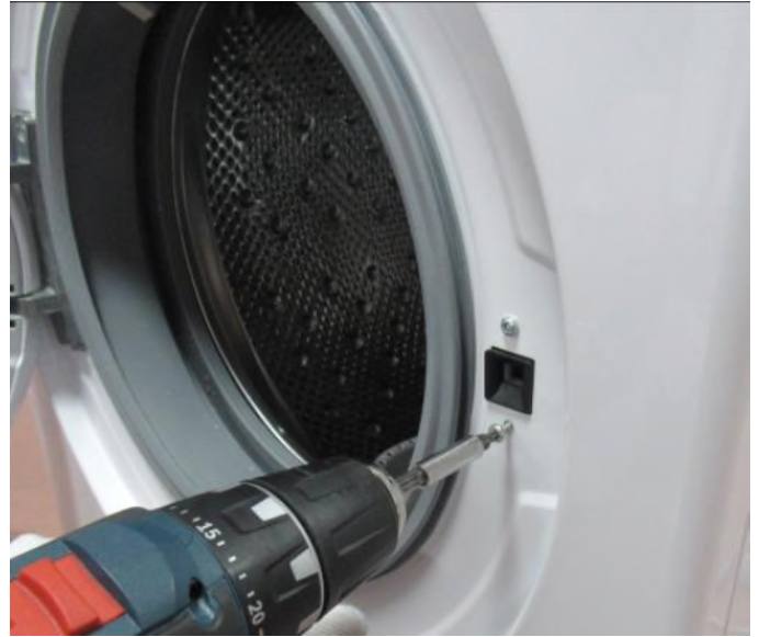
Remove the screws fixing the door lock.
