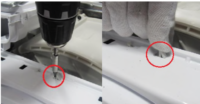
3.7 Remove the screw fixing twinjet elbow.
